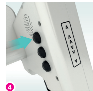
4 Vent contrast using manual keys
