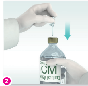
2 Perforate CM and saline containers with spike
